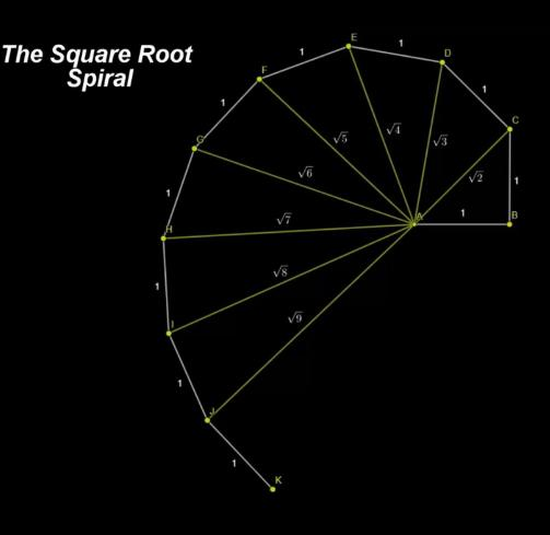
As a result of this construction, the new radius increases, and is equal with the next square root number.
