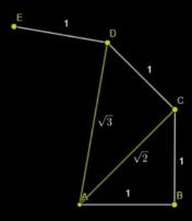
At each step in the development, the spiral is extended with a segment equal with one and perpendicular on the radius in that point.
