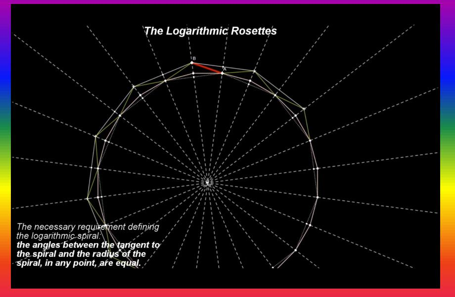
We need to find the location of point **C** such that the angle between **BC** and the radius through **B** is equal with the angle between **AB** and the radius through **A**.
