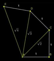
At each step in the development, the spiral is extended with a segment equal with one and perpendicular on the radius in that point.
