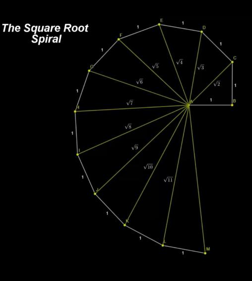
As a result of this construction, the new radius increases, and is equal with the next square root number.
