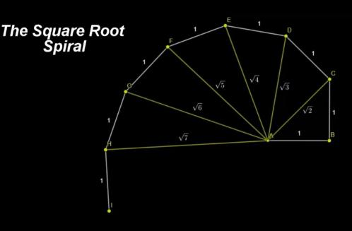
As a result of this construction, the new radius increases, and is equal with the next square root number.
