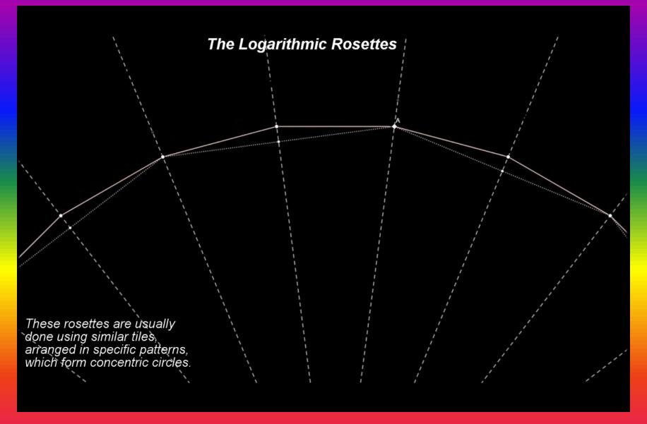
As an example, let's design a logarithmic rosette by starting from a circle approximated by two concentric polygons with 12 sides and respectively 24 sides.
