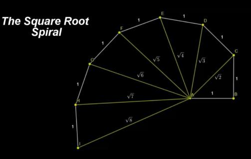
As a result of this construction, the new radius increases, and is equal with the next square root number.
