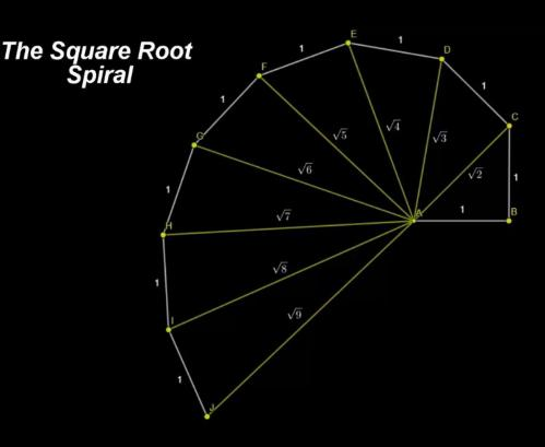
As a result of this construction, the new radius increases, and is equal with the next square root number.
