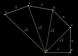
At each step in the development, the spiral is extended with a segment equal with one and perpendicular on the radius in that point.
