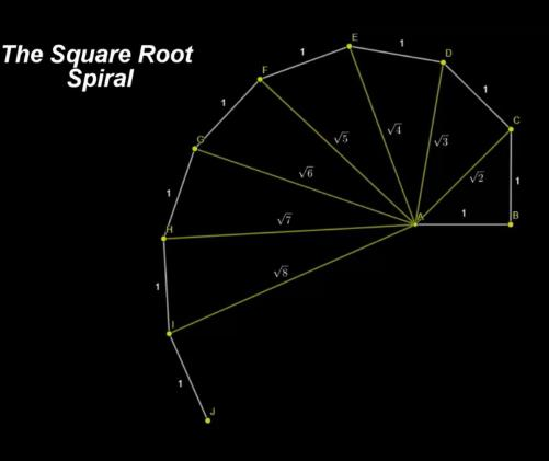
As a result of this construction, the new radius increases, and is equal with the next square root number.
