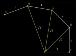
At each step in the development, the spiral is extended with a segment equal with one and perpendicular on the radius in that point.
