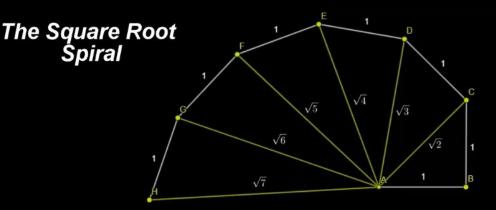
As a result of this construction, the new radius increases, and is equal with the next square root number.
